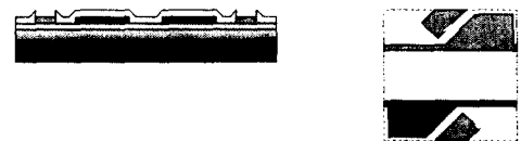
(c) Patterning of oxide and PR removal
