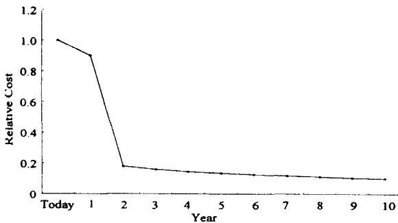
Fig. 3 Relative cost vs. time for a motor and engine of P-HEV
