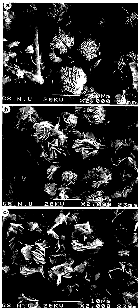
Fig. 2. Scanning electron micrographs of synthetic Na-kenyaite according to reaction time. Molar ratio of reactant mixture: \text{SiO}_2/\text{NaOH} + \text{Na}_2\text{CO}_3 = 10 , \text{H}_2\text{O}/\text{Na}_2\text{CO}_3 = 200 . (a) 48 h, (b) 72 h, (c) 96 h.
