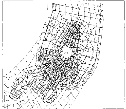
Fig. 5 Recliner part of a seat frame
