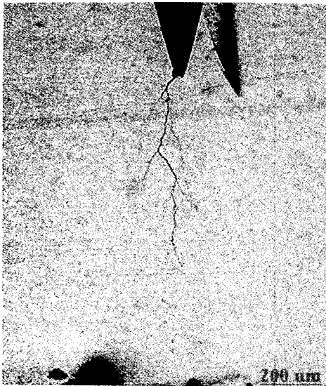
Fig. 3. Electrical treeing deterioration phenomena in the conventional epoxy resin system DGEBA/MDA.
