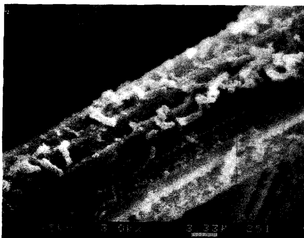
Fig. 4. Scanning electron micrograph of the electrode (anode) in the three-electrode bacteria cultivation system.
