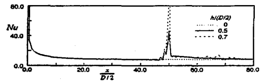
Fig.10 The distribution of the local heat transfer coefficient along the interface of the ice formation for the various heights of stenotic port.
