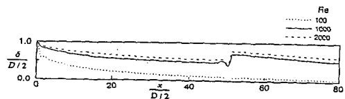
Fig.7 Ice formation layer for various Reynolds numbers in a stenotic tube.
