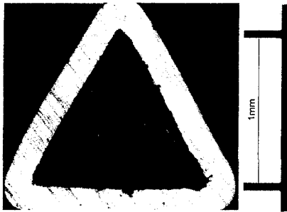
Photo. 1 Microscopic view of cross section of a triangular tube with plane walls obtained by drawing process.
