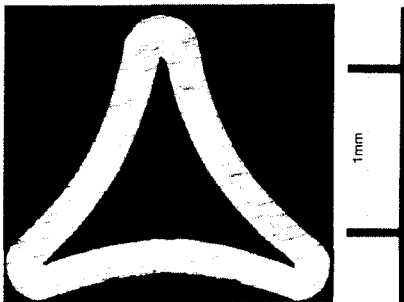
Photo. 2 Microscopic view of the cross section of a triangular tube with curved walls.
