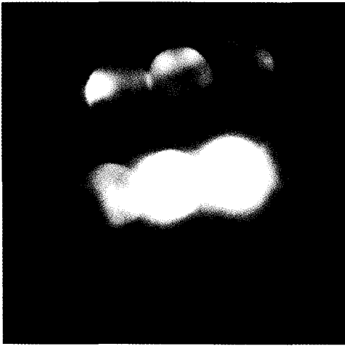
Fig. 8. Micro-diffraction pattern obtained from F1-layer.
