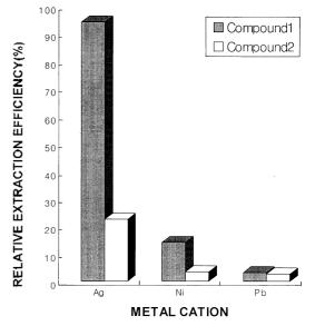
**Figure 3.** Comparative Profile for the extraction of Ag(1), Pb(11), Ni(11) ions in an aquatic environment with N.N-diethyl-2.7-dihexyl-3.6-diazaoetanoic acid (1) and 1.5-bis[2-2'-carboxy-pentadecyloxy) phenoxy]-3-oxapentane (2). Metal aqueous solution =  $3.0 \times 10^{-4}$  M, Organic solution (in chloroform) =  $1.5 \times 10^{-4}$  M, for 30 min, at 30 °C.
