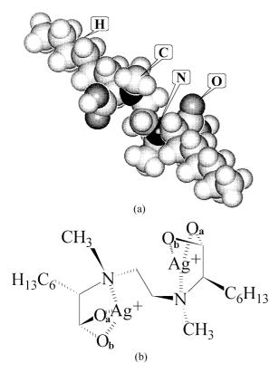
**Figure 2.** Schematic illustration of Energy minimized structure of Ag(I) selective acyclic azapolyether, compound (1): (a) and The structure of the proposed binding of silver ion to compound (1): (b).
