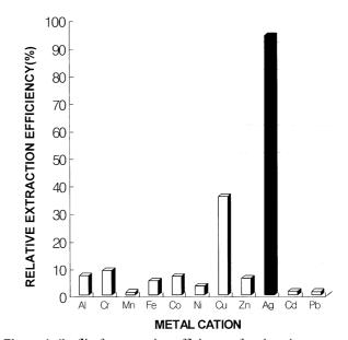
**Figure 1.** Profile for extraction efficiency of various heavy metal ions from aqueous phase into chloroform layer using the compound (1) at 30 °C and pH 6.80. Metal aqueous solution  $-3.0 \times 10^{-4}$  M. Organic solution (in chloroform) =  $1.5 \times 10^{-4}$  M.
