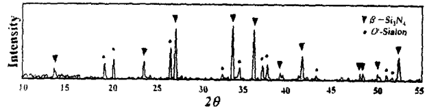
Fig. 7. X-ray diffraction profile of GPSed Si 3 N 4 body at 1950°C, nitrided at 1470°C.
