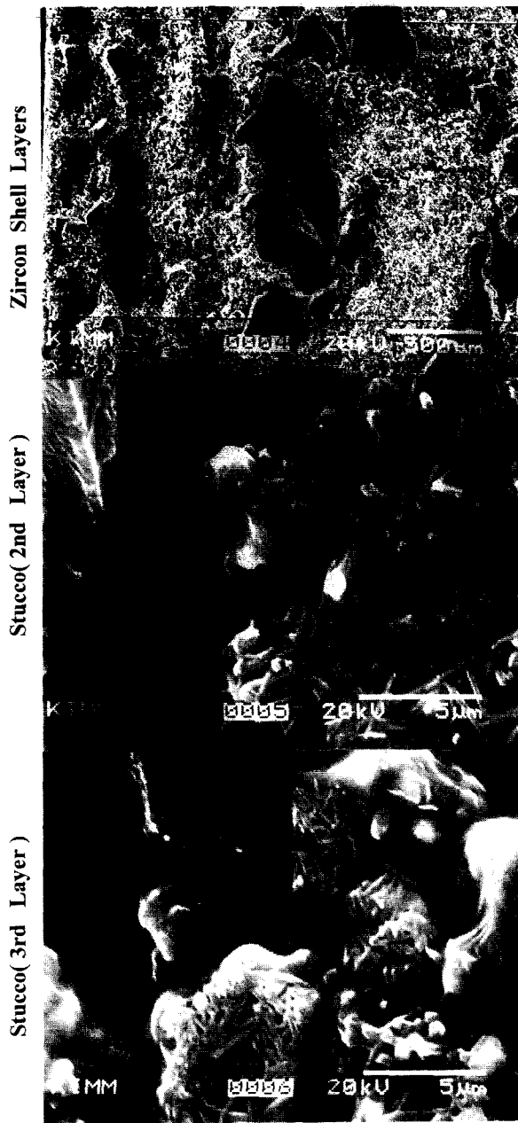
Fig. 11. Cross sectional micrographs of the dip-treated zircon-based shell mold sintered at 1500°C for 5 hrs.
