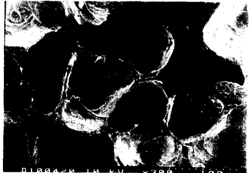
Fig. 8 SEM photography=Aquacell: Water+CO 2 Foamed PMMA at 80℃, 30s-saturated at 4.48MPa 30℃
