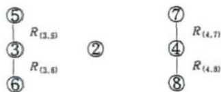
Fig. 6 Graphical representation of the bogie system
