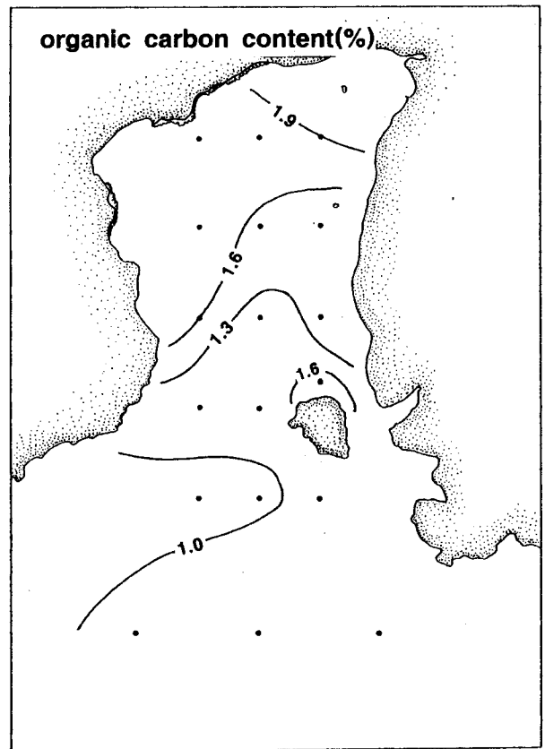
Fig. 3. Spatial distribution of organic carbon content (%) of the surface sediment in Aenggang Bay, January 1995.
