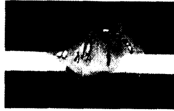
(b) The appearance of bead with blow holes
