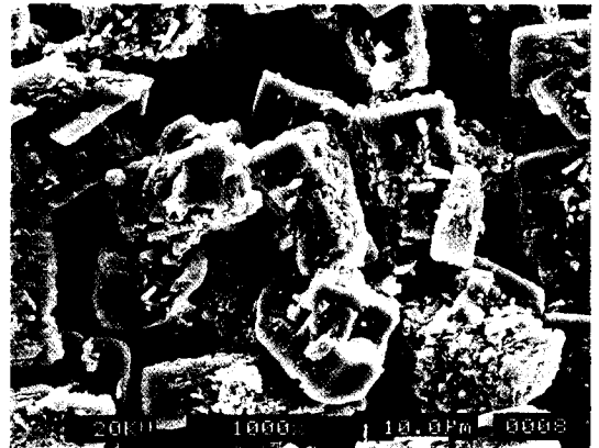
Fig. 2. SEM micrograph of calcium hydrogen phosphate obtained at pH of 6.2, temp. of 80°C and time of 24 hrs.
