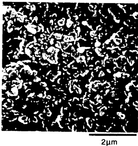
Fig. 4. SEM photographs of surface deposited on the WC substrate in H 2 -10%CH 4 .
