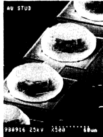
Fig. 1. Scanning electron microscopy of coined Au stud bumps formed on Al pads of test chip.
