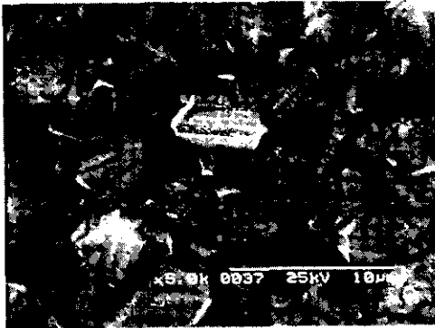
Fig. 3. SEM image of Cu deposited surface of undoped diamond films. Cu was electroplated from CuSO 4 solution for 15min.
