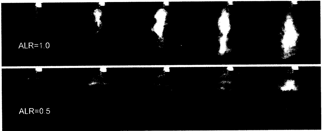
Fig. 5 Spray development of the AAFI. P_{sup} = 0.7\text{MPa} , P_{amb} = 0\text{MPa} . Time interval is 1ms
