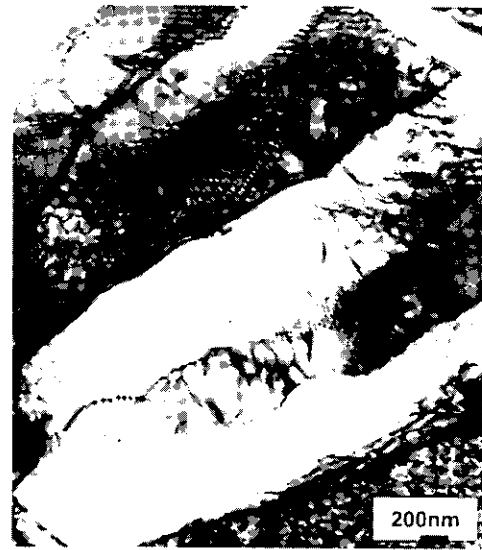
Fig. 8. TEM micrograph of \beta -quenched specimen showing dislocation rearrangement as recrystallization progresses
