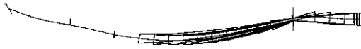
Fig 3 First horizontal mode in the global y direction of the model for the two linked bridges (plan view)
