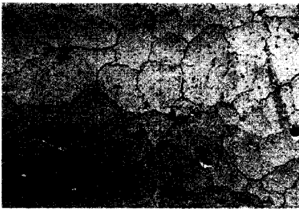
Unit contents of expansion admixture 80 \text{ kg/m}^3
