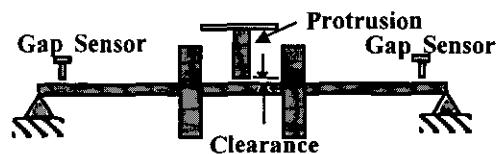
Fig. 1 Schematic diagram of experimental apparatus for partial rubbing
