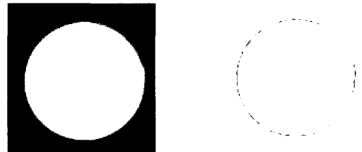
(a) An image obtained from the CCD camera (b) The boundary extracted from the original image.
