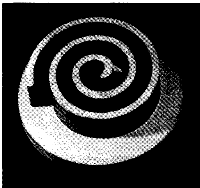
Fig. 10 The non-symmetric rotating part manufactured by back-pressure forming
