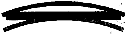
Fig. 6 Schematic view of bending process for bumper rail. 1. Upper die 2. Workpiece 3. Lower die
