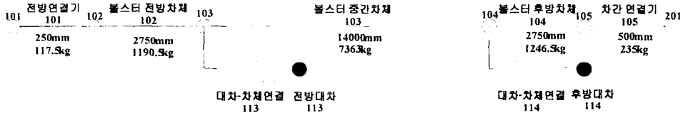
Fig. 2 One-dimensional model of the TC-car
