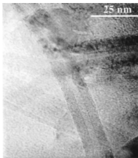
Fig. 2. TEM micrograph of MWNTs synthesized under helium pressure of 360 torr.
