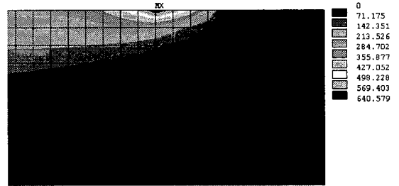
Fig. 3 Temperature distribution in insulated elastic half-space, with uniform heat source
