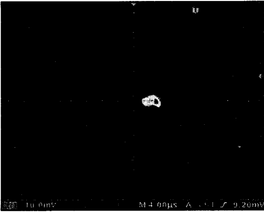
Fig. 15 Lissajous loop above critical speed with ADB (at 1950.2 rpm)
