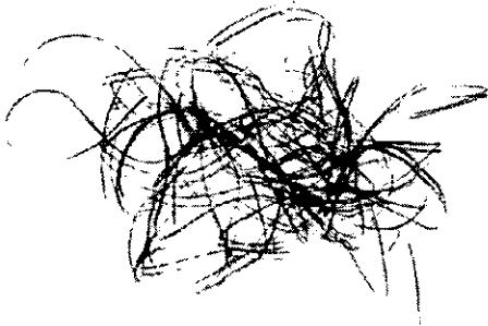
Fig. 9 Photo of Chip in 0.160mm/rev without Chip Control
