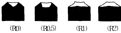
Fig. 10 Schematic diagram of failure plane for the radius of notch tip at -30°C, 0°C, 20°C
