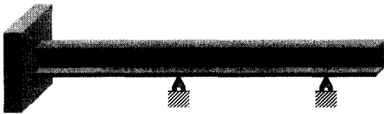
Fig. 4 Numerical model 2: channel section beam
