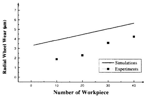
Fig. 6 Comparison of prediction and experimental result for grinding wheel wear
