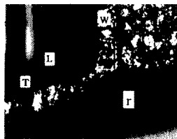
Fig. 14 Parameters(W, T, L) of drill exit-step( #3 )
