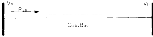
Fig. 7 Active power between two buses
