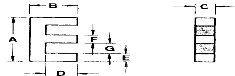
Fig. 3 R-47228EC core(mm): A=72.4, B=27.9, C=19, D=17.8, E=9.53, F=19, G=16.9
