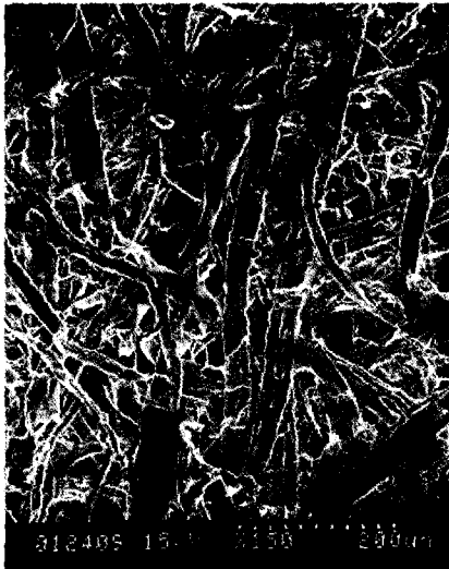
Fig. 10. SEM photomicrograph of Sangguhyung on top side (×150).
