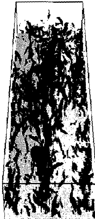
Fig. 4 Turbulent eddies in Reynolds number=300 channel flow. Vortices that are part of a hairpin packet have been highlighted to make them visible amongst the background clutter. Note the similarity between the groups of eddies in this fully turbulent flow and the complex hairpin packet in Fig. 3
