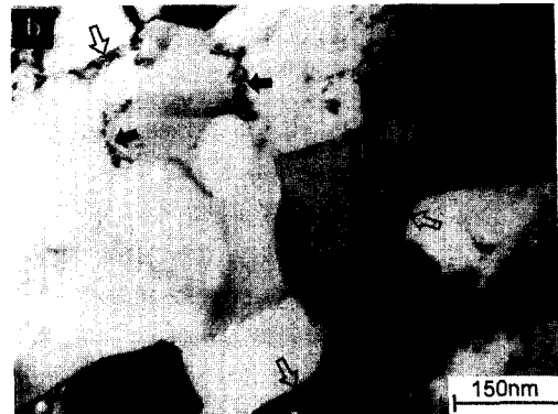
Fig. 5. TEM micrographs of a longitudinal (a) and transverse (b) sections of Cu-Nb heat-treated at 500°C showing spheroidized or split niobium filaments.
