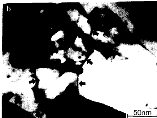
Fig. 3. Longitudinal (a) and transverse (b) TEM micrographs of Cu-Nb annealed at 400°C. Dislocation arrays are labeled, "A", dislocation networks are labeled "N".
