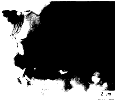
Fig. 6. TEM micrograph of the \text{Fe}_{0.98}\text{Co}_{0.02}\text{Si}_2 compacts, showing fully transformed \beta - \text{FeSi}_2 after isothermal annealing.
