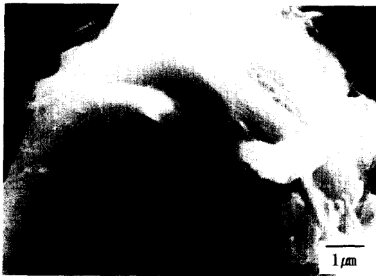
Fig. 13. SEM micrograph showing the surface morphology of SiCp extracted from SiCp/2024Al.
