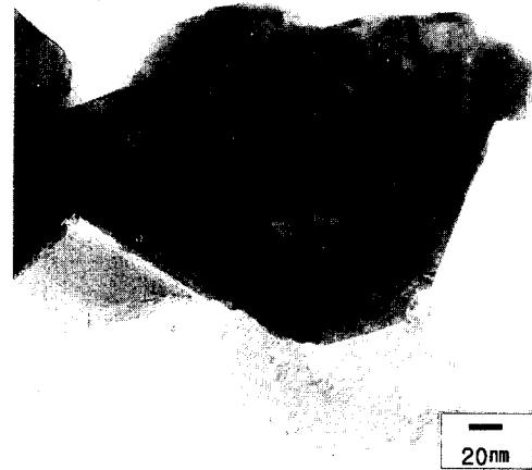
Fig. 9. TEM micrographs of powders calcined at 800℃.
