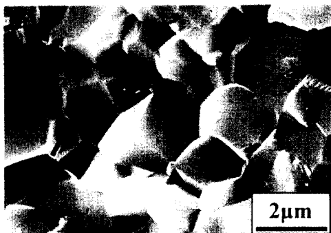
Fig. 8. Fracture surface of the hot-pressed specimens observed in SEM; a) monolithic Al 2 O 3 , b) Al 2 O 3 /10 wt% Fe-Ni composite.
