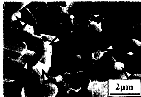
Fig. 8. Fracture surface of the hot-pressed specimens observed in SEM; a) monolithic Al 2 O 3 , b) Al 2 O 3 /10 wt% Fe-Ni composite.
