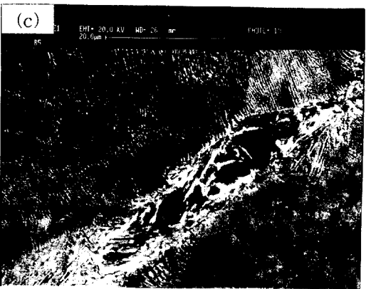
Fig. 3. Cross sectional SEM of laser surface hardened 40Cr steel regions from top to bottom(power 1400W, scanning velocity 27mm/sec) (a) Top (b) Middle (c) Bottom
