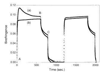
Figure 6. Growth and relaxation curves of birefringence: (a) the sample 1 (upper curve) and (b) the sample 2 (lower curve). At point A, the linearly polarized laser (pump beam) is turned on: at point B, the pump beam is turned off: at point C the circularly polarized laser (erasing beam) is turned on.
