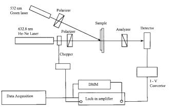
Figure 5. Schematic diagram of optic set-up for investigating photo-induced birefringence of film.
