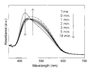
**Figure 4**. Spectral change of the sample 1 on exposure to 532 nm laser at some time intervals: 532 nm laser was on for 0, 1, 2, 3, 5, 18 mins (solid) and 5 mins after 532 nm laser was off (dash).
