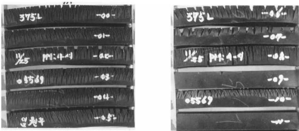
Figure 8. Ozone resistance according to various rubber composition for specimen-A.
