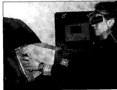
Fig. 6 Portable inspection of composite fuselages
